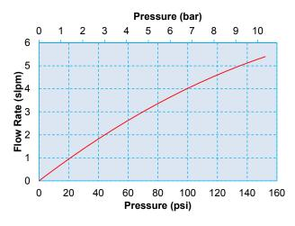
Model 2 - 0.020" (0.51 mm) Orifice Pressure (bar)
