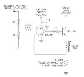
This simple current driver circuit draws only 1 mA at the input control (0-5VDC) and provides control for any VSO® valve configuration regardless of valve voltage or resistance.
