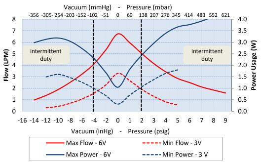
The above graphs represent examples of performance for the pumps series handling air at 800 feet (244M) above sea level at 75° F (24° C). Performance will vary depending on barometric pressure and media temperature.
