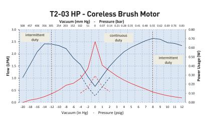
The above graphs represent examples of performance for the pumps series handling air at 800 feet (244M) above sea level at 75° F (24° C). Performance will vary depending on barometric pressure and media temperature. Curves are representative of standard pump configurations. Pump configurations could be customized for higher or lower flows, depending on specific customer requirements.
