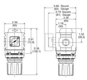
Inches (mm) NOTE: 1.90 in. (48mm) hole required for panel nut mounting.
