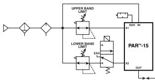
Note: For valves with normally open solenoids, reverse the X1 and X2 connections.
