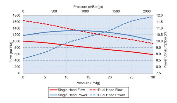
Typical flow performance is shown with standard high flow configurations with barb ports and brushless DC motor. Performance will vary depending on port and motor selection. Please contact Parker for the typical flow performance for a specific part number and configuration.
