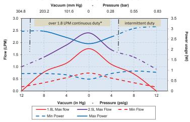
The above graphs represent an example of performance for the pump series handling air at 800 feet (244 m) above sea level at 75°F (24°C). Performance will vary depending on barometric pressure and media temperature. A variety of configurations can be accommodated to meet application requirements. Curves are representative of standard pump configurations. Pump configurations could be customized for higher or lower flows depending on specific customer requirements.
