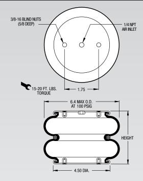
NOTE: A bead plate part is shown. This part is also available with bead rings. Bolts are not included. See pages 8-10 for explanation.
