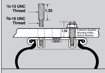
If a protruding bolt rather than a blind nut is preferred to attach the air spring, a STUD ADAPTER is available from Firestone:
