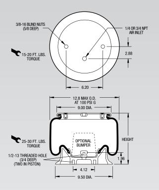
NOTE: Bellows will not compress properly with less than 10 PSIG internal pressure.
