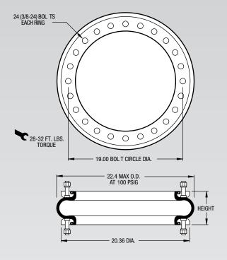
NOTE: A bead ring part is shown. This part is also available with rolled plates. See page 11 for explanation.
