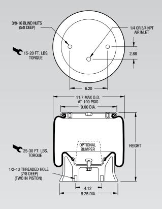
NOTE: Bellows will not compress properly with less than 10 PSIG internal pressure.
