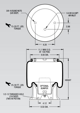
NOTE: Bellows will not compress properly with less than 20 PSIG internal pressure.
