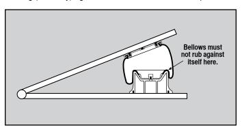
NOTE: The max and min height are not the vertical distance but the actual distance the bellows moves with the angle.
