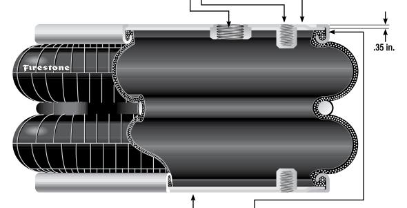
**CLAMP RING** This ring is crimped up under the bellows bead to permanently attach the bead plate to the bellows. It is also zinc/chromate plated for rust protection.
