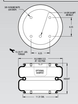
NOTE: The bellows extends beyond the bead plates at minimum height.
