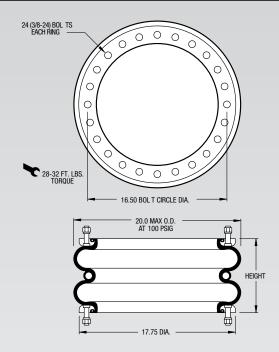
NOTE: A bead ring part is shown. This part is also available with rolled plates. See page 11 for explanation.
