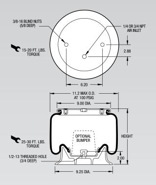
NOTE: Bellows will not compress properly with less than 10 PSIG internal pressure.
