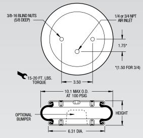
NOTE: A bead plate part is shown. This part is also available with bead rings. See pages 8-10 for explanation.
