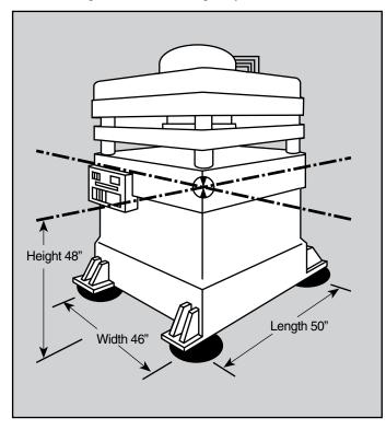
In the above example, the most narrow distance between two Airmounts is 46 inches The height to the c.g. is 48 inches; therefore, this system does not meet our guideline. Two possible solutions would be:
