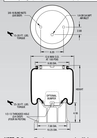
NOTE: Bellows will not compress properly with less than 10 PSIG internal pressure.
