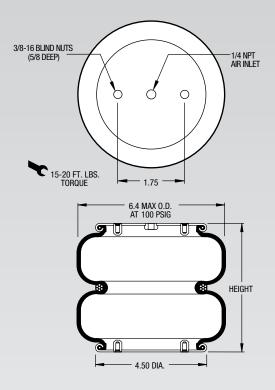
NOTE: A bead plate part is shown. This part is also available with bead rings. Bolts are not included. See pages 8-10 for explanation.
