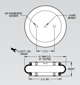
NOTE: A bead plate part is shown. This part is also available with bead rings. See pages 8-10 for explanation.
