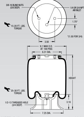
NOTE: Bellows will not compress properly with less than 10 PSIG internal pressure.
