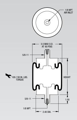
NOTE: This Airstroke actuator must be guided throughout the stroke.
