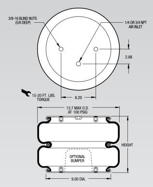
NOTE: The bellows extends beyond the bead plates at minimum height.
