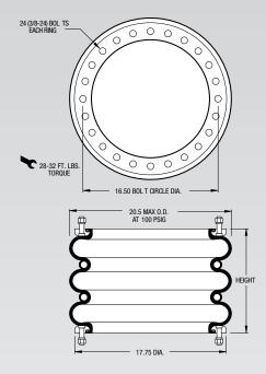
NOTE: A bead ring part is shown. This part is also available with rolled plates. See page 11 for explanation.
