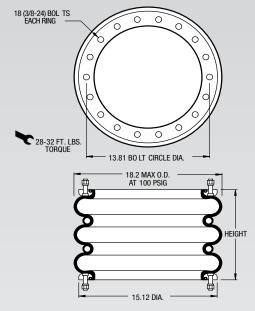
NOTE: A bead ring part is shown. This part is also available with rolled plates. See page 11 for explanation.
