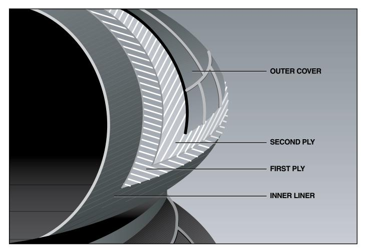
An air spring is a carefully designed rubber/fabric bellows which contains a column of compressed air. The rubber bellows itself does not provide force or support load. This is done by the column of air.
