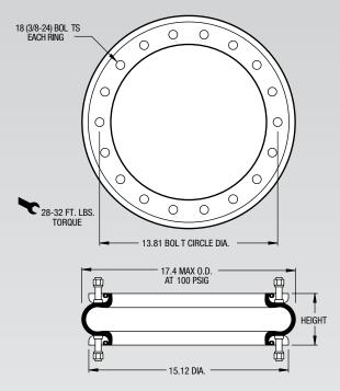
NOTE: A bead plate part is shown. This part is also available with rolled plates. See page 11 for explanation.
