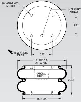
NOTE: A bead plate part is shown. This part is also available with bead rings. See pages 8-10 for explanation.
