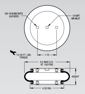
NOTE: A bead plate part is shown. This part is also available with bead rings. Bolts are not included. See pages 8-10 for explanation.
