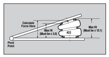
Reversible sleeve Type 1T parts may also stroke through an arc. In this case, care must be taken to prevent the bellows from rubbing (internally) against itself where it rolls over the piston:
