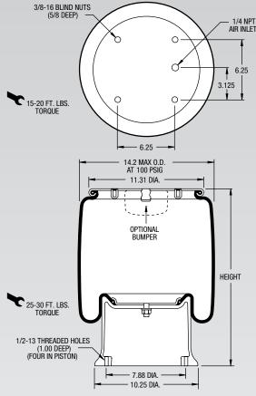
NOTE: Bellows will not compress properly with less than 20 PSIG internal pressure.
