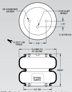
NOTE: The bellows extends beyond the bead plates at minimum height
