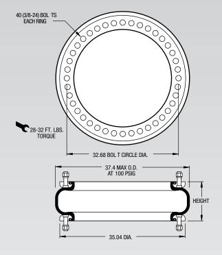
NOTE: The effective length of the 1 7/8 bolt is 1.05" in this bead ring.
