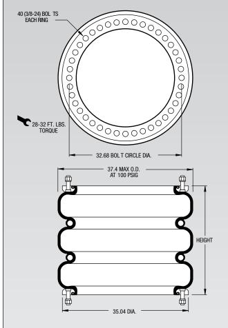
NOTE: The effective length of the 17/8 bolt is 1.05" in this bead ring.
