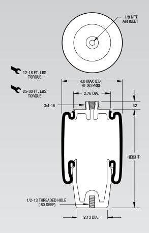
NOTE: Bellows will not compress properly with less than 10 PSIG internal pressure.
