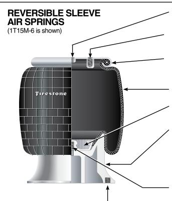
**THREADED HOLE** May be used for attachment to mounting surface. Not included in some pistons (See individual data sheets for specific part configuration.)
