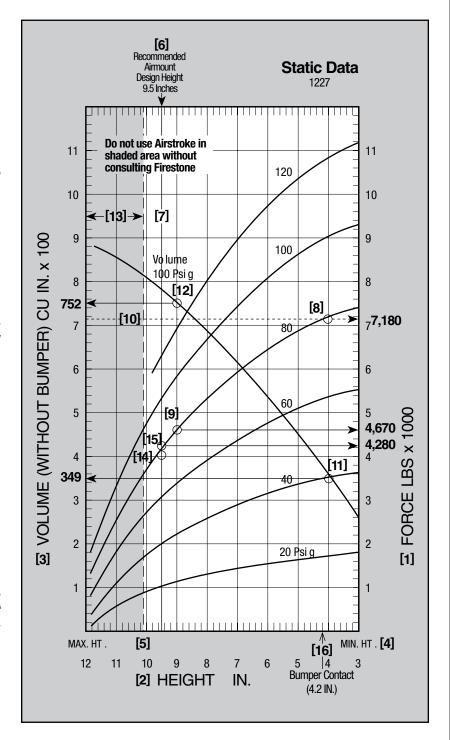
In the example the effective area of a #22, at 4.0 inches using the 80 psi curve, is:
