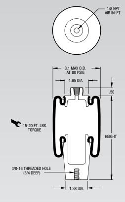
NOTE: Bellows will not compress properly with less than 10 PSIG internal pressure.
