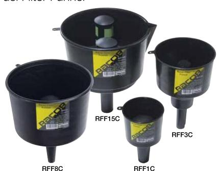
Caution for Users: Petroleum products flowing over a plastic surface generate static electricity. Caution should be taken to ensure that the RFF is grounded to reduce static electricity buildup and reduce the chance of explosions or fire. Electrically bond the funnel by using a wire with a metal clip on each end and clamp one to the upper rim of the funnel and the other to the fueling source. For example, the metal gas can or nozzle from the pump.
