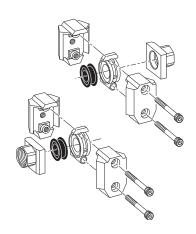
Port block connectors allow you to make threaded port connections to modular units and are available in various port sizes to match your system requirements.
