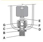
Oil enters the unit at the pipe thread fitting (A) with a supply pressure that is a minimum of 20 psig above the lubricator air pressure. With the float lowered, oil flows through metering orifice (B) and lifts the check ball (C). Oil continues to flow past the shuttle chamber annulus (D) and out the cross drilled hole (E). As the
