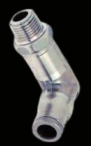
Parker Legris has developed 2 ranges of stainless steel fittings (LF 3800 or LF 3900 in full 316L) for conveying corrosive fluids in aggressive environments. These ranges provide two complementary levels of corrosion resistance and a hygienic external design.
