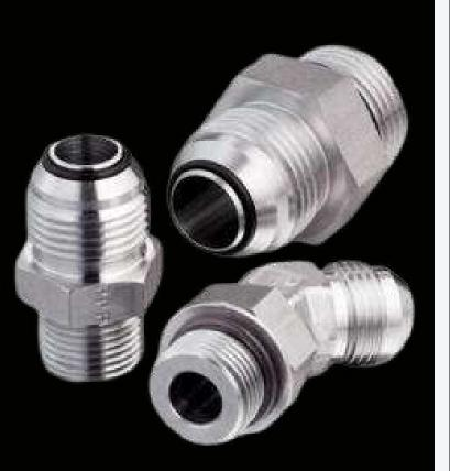
The appeal of the 37° flare fitting is in its simplicty, compact design, ease of assembly, reliability, wide availability and acceptance. It is especially suited for low and medium wall thickness tubing. Suitable for pressures up to 500 bar for small sizes and up to 140 bar for the largest sizes.
