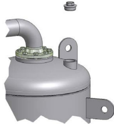
Unscrew the sleeve plug
