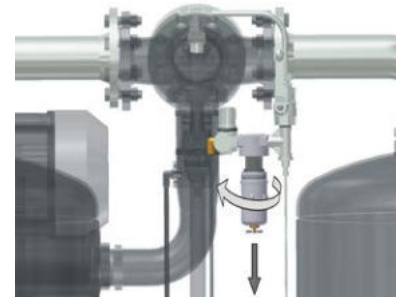
Open control air filter
