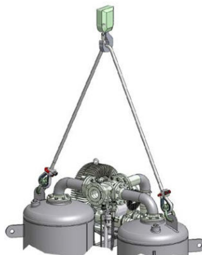
Transport by crane
