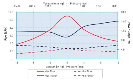
The above graph represents an example of performance for the pumps series handling air at 800 feet (244m) above sea level at 75°F (24°C). Performance will vary depending on barometric pressure and media temperature. Curves are representative of standard pump configurations. Pump configurations could be customized for higher or lower flows, depending on specific customer requirements.
