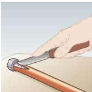
1. Cut lengthwise along a line at approximately a 20 angle from centre line of hose. The cut should be approximately 1" long. Be careful not to nick barbs when cutting the hose.
