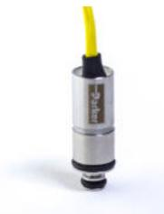
The Series C7 is a miniature cartridge style solenoid valve with a compact 7 mm diameter. This unique design combines small size, light weight and low power consumption with high flow repeatability and fast response time over an exceptionally long life, up to 130 million cycles. Available in 2-way and 3-way configurations, the valve is manifold mounted utilizing a simple securing system reducing assembly time.
