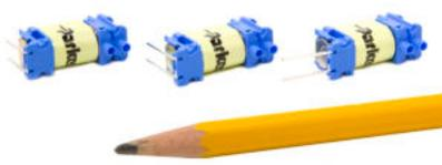
The Series LX-Valve is a miniature latching pneumatic solenoid valve measuring only 8 mm in width. The compact size, light weight, and power saving latching feature of the Series LX-Valve is the ideal solution for portable/battery powered applications. The body construction of the Series LX-Valve is suited for manifold or barbed-tube pneumatic connections and is available in a 2 way configuration.
