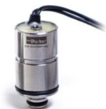
The Series C15 is a miniature cartridge style solenoid valve with a unique design that combines small size, light weight and low power consumption with high flow repeatability and fast response time over an exceptionally long life, up to 500 million cycles. Available in 2-way and 3-way configurations, the valve is manifold mounted utilizing a simple securing system reducing assembly time.
