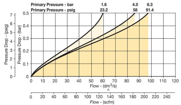
**Popular Combinations:** Inlet pressure 145 psig (10 bar), secondary pressure 91.3 psig (6.3 bar), 14.5 psig (1 bar) pressure drop.
