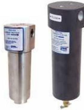
FFC series filters are designed to protect critical engine components in CNG powered vehicles. Contaminants can be introduced into a vehicle's fuel tank when being fueled or may come from compressors and/or storage facilities. A grade 6 coalescing filter is specifically designed to remove oil, water, and solid contamination from compressed natural gas.
