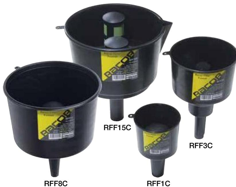
Racor Filter Funnel (RFF) is a heavy-duty, fast-flow, filter-in-a-funnel that separates damaging free water and contaminants from gasoline, diesel, heating oil, and kerosene.
