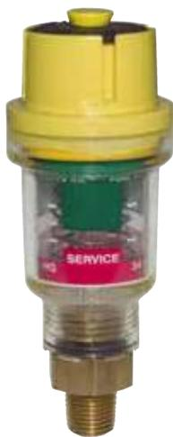
Vacuum restriction indicators monitor element condition as the filter slowly becomes clogged with contaminants. As the element gets dirty, restriction increases and less fuel is delivered to your engine causing the engine to lose power and eventually stall. By installing a vacuum indicator in your fuel system, visual monitoring of element condition is possible at a glance, increasing fuel system troubleshooting efficiency, eliminating guess work, and lengthening element change intervals.
